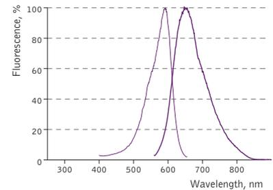
**TurboFP650 normalized excitation (thin line) and emission (thick line) spectra.**
