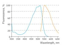
KillerOrange normalized exitation – blue line (em@600 nm) and emission – orange line (ex@510 nm) spectra.
